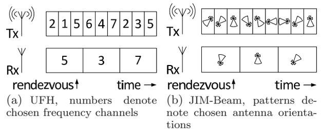
Figure 1: Illustration of UFH and JIM-Beam
