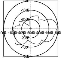
Figure 2: Radiation pattern of antenna
