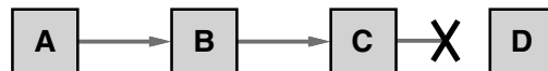
Figure 2: An example of DSR Route Maintenance. When forwarding a packet from node A to node D, node C detects that the next link along the source route (the link from C to D) is broken and returns a ROUTE ERROR to node A, the original sender of the packet.
