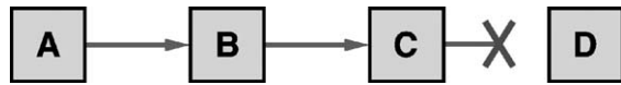
Figure 2. Example of DSR Route Maintenance, in which intermediate node C detects a broken link to D when forwarding a packet from source node A .
