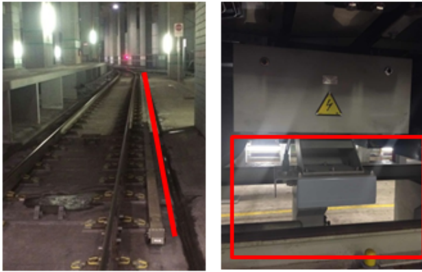
Fig. 1. Leaky waveguide deployment in railway systems (left) and the corresponding trainborne antenna (right)
