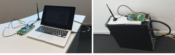
Figure 8: Device setup for the experiments (left) and device setup for the repeater node (right).
